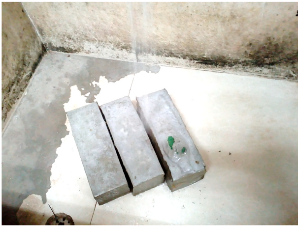
Fig. 8. Three plastic brick samples after removing from the cardboard case and completion of curing period of 14 and 28 days with a similitude like the normal clay brick.
