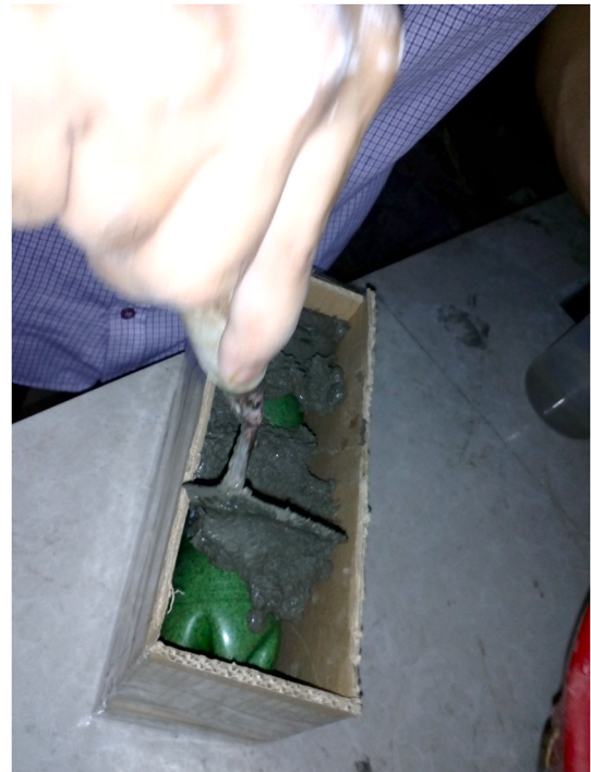
Fig. 7. Preparing a plastic brick sample with blended mortar cast in the cardboard frame and the PET plastic bottle set in the center.
