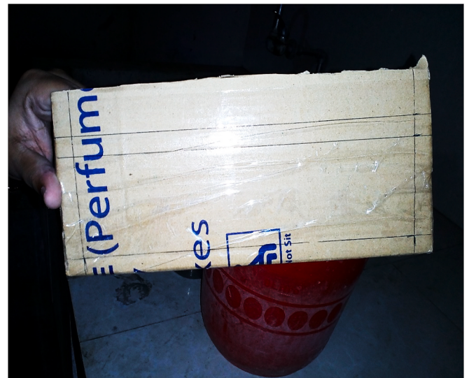
Fig. 6. Casing prepared by using a cardboard box with dimensions selected as (L \times B \times H = 9.5 \text{ in} \times 3.5 \text{ in} \times 3.0 \text{ in}) .
