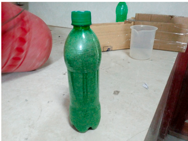
Fig. 5. A sample 500 mL waste PET plastic bottle fully compacted with sand as the filler material and tightly sealed with a cork.
